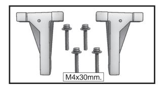
Mark and drill 4 holes for engine mount. Insert 4 blind nuts to firewall.
