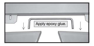
Glue the elevator hinges in place using the same techniques used to hinge the ailerons.
